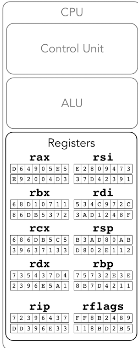
Figure 1-3. Approximation of Intel 64: general purpose registers
